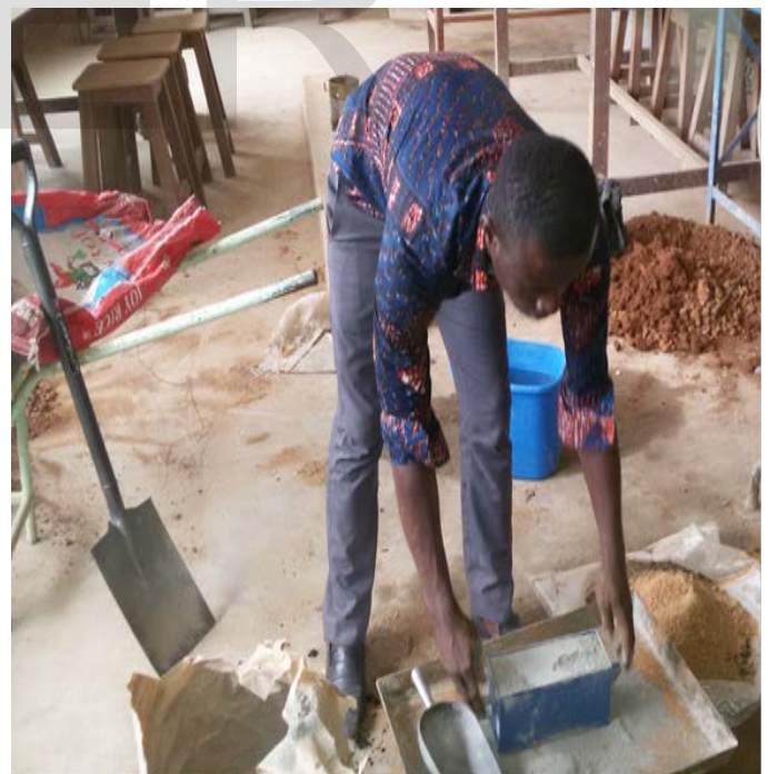
Fig 1: Batching of materials for block samples
