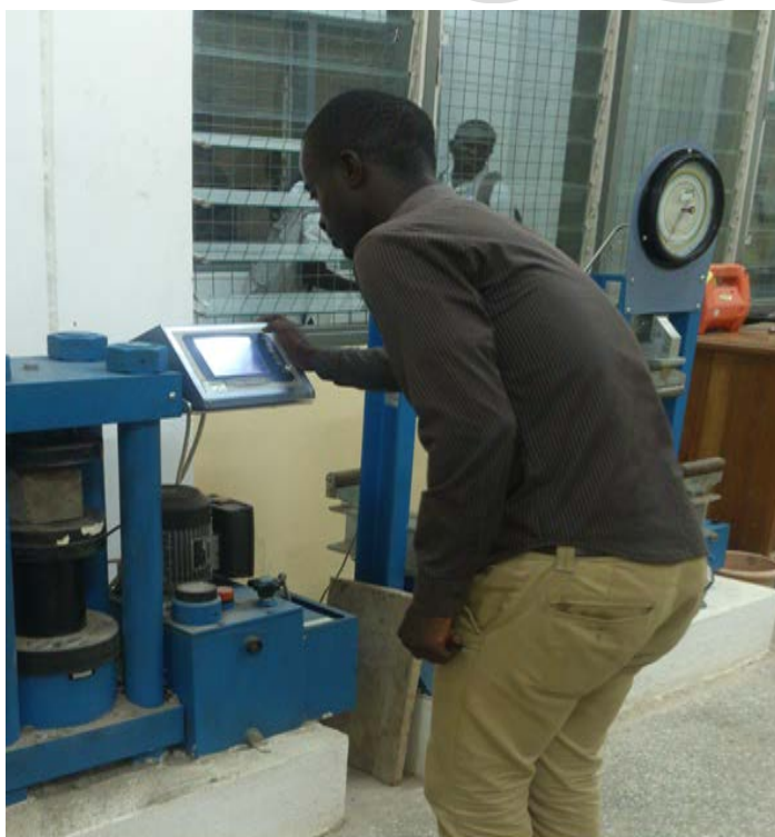
Fig 2: Crashing of Blocks samples
